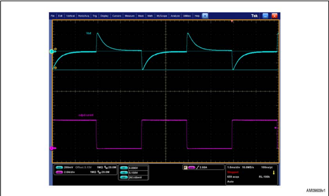
Figure 26. Response of the converter to a 2 A - 4 A load transient
